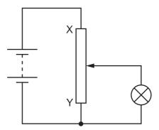
What happens to the brightness of the lamp and the potential difference (p.d.) across the lamp, when the slider is moved from X to Y?
