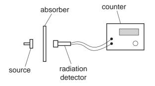
When a piece of paper is used as the absorber, the count rate drops to the background count rate.
